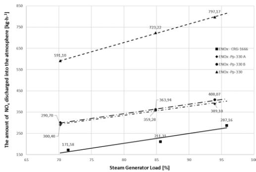
Fig. 10. The Amount of NO<sub>x</sub> Discharged
